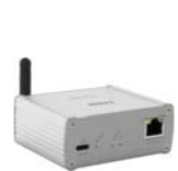
eLAN-RF-103 Smart RF gateway with LAN
